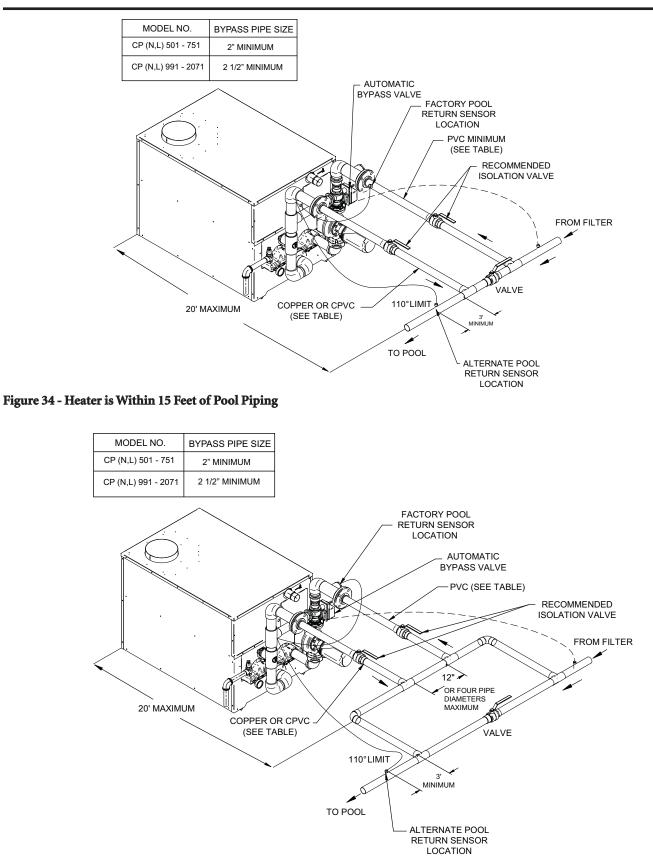
Figure 35 - Heater is Beyond 15 Feet of Pool Piping
